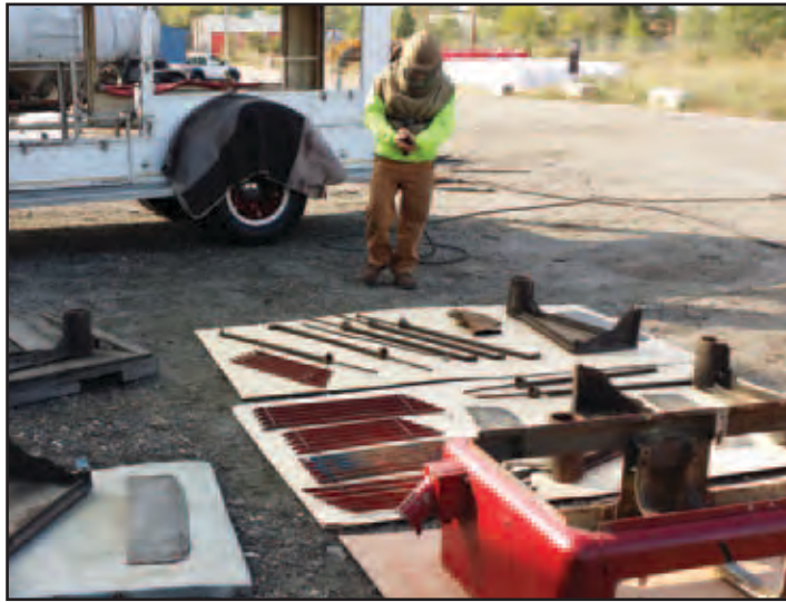
L: Sandblasting the cradle assembly.
