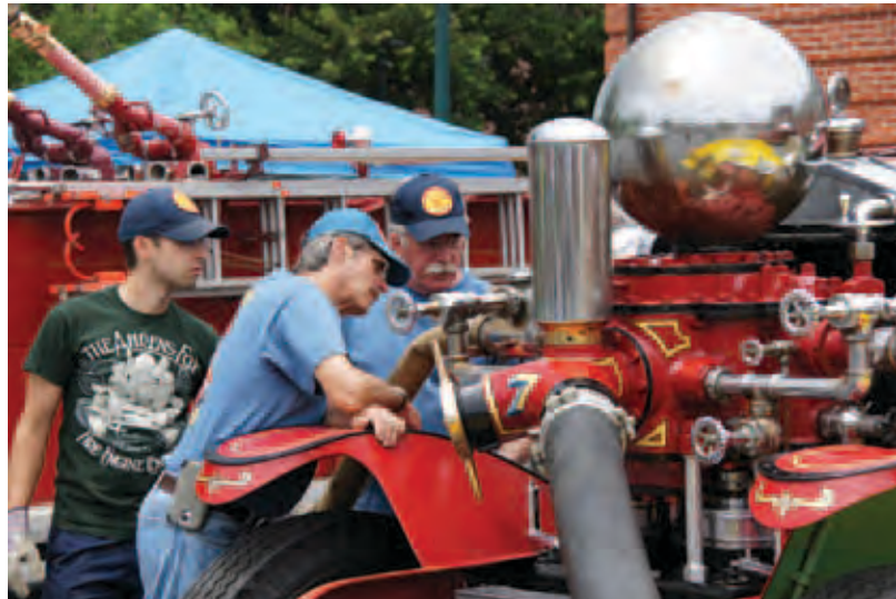
Ahrens-Fox of Cincinnati specialized in making motor pumping cars with piston pumps. This technology was closest to what fire fighters had known for two hundred years. It was the most efficient machine but it was also the most complicated to make. The Museum's 1922 Fox is seen here pumping at the Harrisburg Fire Museum in June. l to r: Alex Guerrieri, Dennis Crawford, Steve Heaver.
