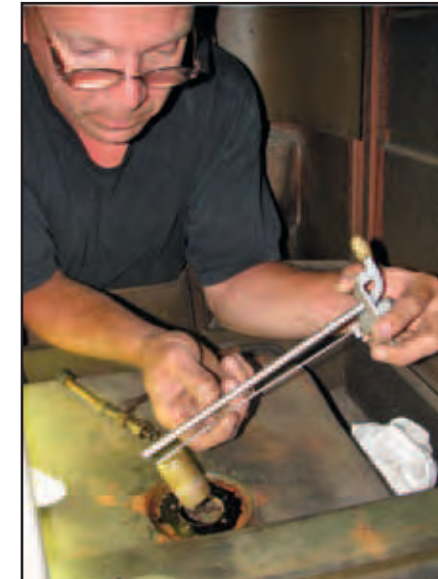
L: Brian works on the fuel gauge sending unit.
